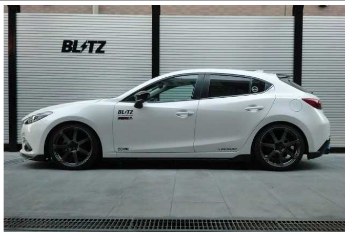
Front: -40mm down / Rear: -45 mm down ※The image is AXELA Sports (BM2FS).
