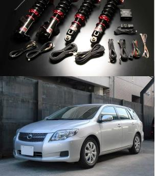
• The damping force can be easily adjusted from a controller inside your vehicle (Choose from 96/64/32 levels of adjustment). By utilizing a stepping motor, a maximum of 96 levels of adjustment is possible to finely tune the vehicle setup for your desired ride quality.
