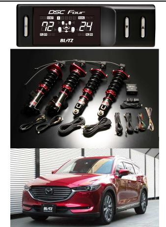
• The damping force can be easily adjusted from a controller inside your vehicle (Choose from 96/64/32 levels of adjustment). By utilizing a stepping motor, a maximum of 96 levels of adjustment is possible to finely tune the vehicle setup for your desired ride quality.
