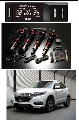
•The damping force can be easily adjusted from a controller inside your vehicle (Choose from 96/64/32 levels of adjustment). By utilizing a stepping motor, a maximum of 96 levels of adjustment is possible to finely tune the vehicle setup for your desired ride quality.
