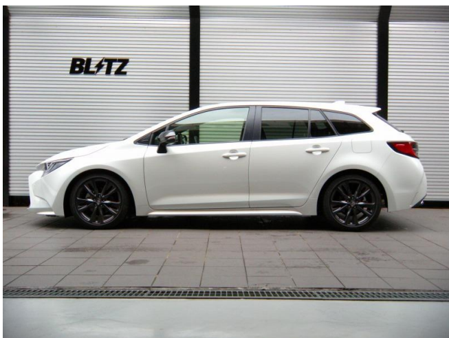
Front: -33mm Down / Rear: -26mm Down
