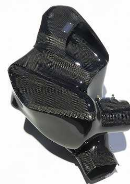
27026_CARBON INTAKE SYSTEM DB42 SUPRA
