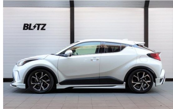
Front : -36mm Down / Rear : -50mm Down
