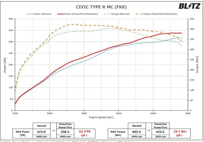
$\odot$  Increase in Maximum Output 22.3PS , Increase in Maximum Torque 19.1Nm
