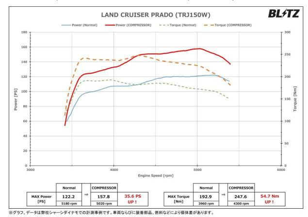
OMaximum Horsepower Increase of 35.6PS. Maximum Torque Increase by 54.7Nm.
