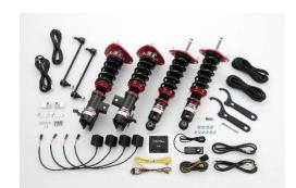
$\ensuremath{\mbox{\%}}\mbox{AT/MT}$  compatible, Trunk Side panel must be modified for proper installation.
