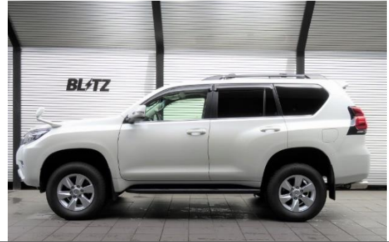
Front : +59mm(2.3in) Up / Rear : +25mm(0.9in) Up
