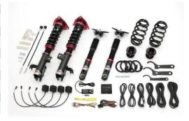
■ Remarks : Rear damping force adjustment dials are located inside the wheel well. ※Abbreviation for Spring Types 「ST:ID62 Straight Spring」, 「BS:Barrel or Tapered, Vehicle Specific Springs」 \*Adjustability in ride height may vary between vehicles.
