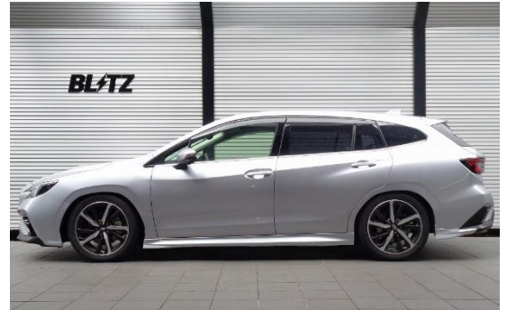
Front : -35mm Down / Rear : -27mm Down
