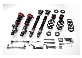
■ Remarks: Includes Canceler. Installable on vehicles equipped with adjustable damping force. However, you will not be able to adjust the damping force using the vehicle electronics. Rear damping force dial located inside the wheel well.
