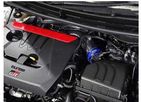
SUCTION KIT BLUE Installation Example
