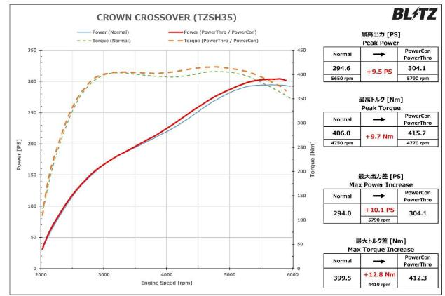
O Crown Crossover: Increase in Maximum Output 9.5PS . Increase in Maximum Torque 9.7Nm
