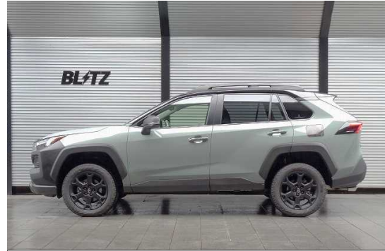
Front : +29mm(1.1in) Up / Rear : +26mm(1.0in) Up
