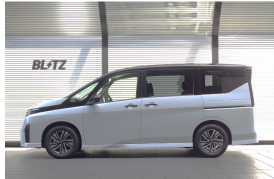
Front : 43mm Down / Rear : 30mm Down
