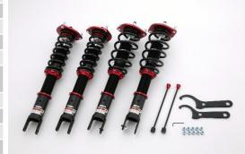
■ Remarks: MT/AT Compatible. The rear trunk must be modified to install damping force extension dials.
