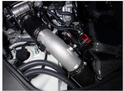
GT-R NISMO R35 Release Type Installation Example
