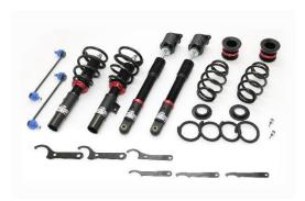
■ Remarks: Compatibility checked for HYBRID model. FL1 (AT) Unchecked. Rear damping force dials located inside wheel well.
