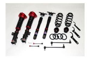
■ Remarks: Only for 300e. Metals panels above front upper mount must be drilled to allow access to the damping force extension dials. Rear damping force dials located inside wheel well. DSC PLUS is recommended.
