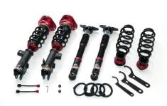
■ Remarks: 4WD Only. Metal panels above upper mount must be modified for proper installation. Rear damping force adjustment dials located inside wheel well. DSC PLUS recommended. Ride height data from MXGH15.
